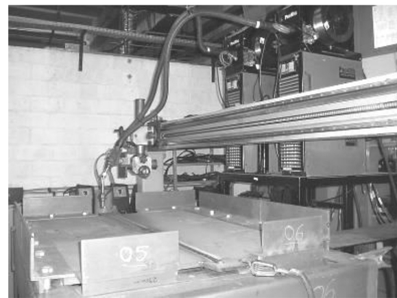
Fig. 2 Plates fixed by clamps along the edges on the support table and automatic double-electrode welding machine.
